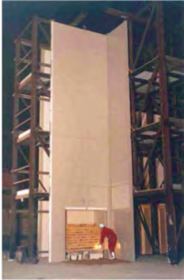
Fig. 7.3 BS8414-2 test rig (from BRE report BR135 [17])
